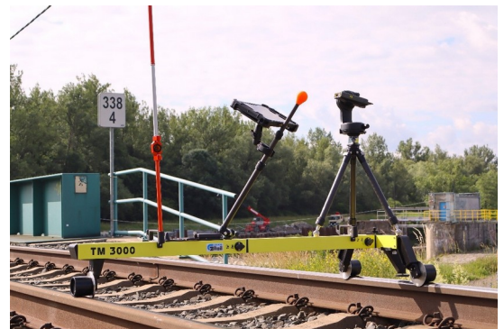
TM3000 with prism and Leica DISTO X6 on the tripod mount
